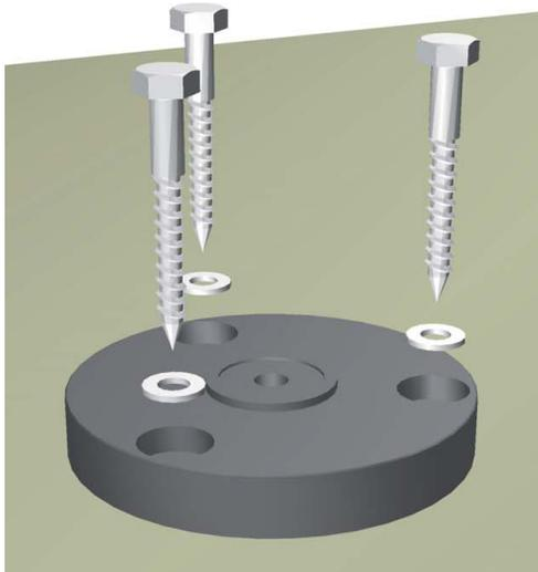
The central plate for the rotor must be secured with 3x  $\Phi 12$  screw plugs, washers and 10x80mm hexagon-head bolts.
